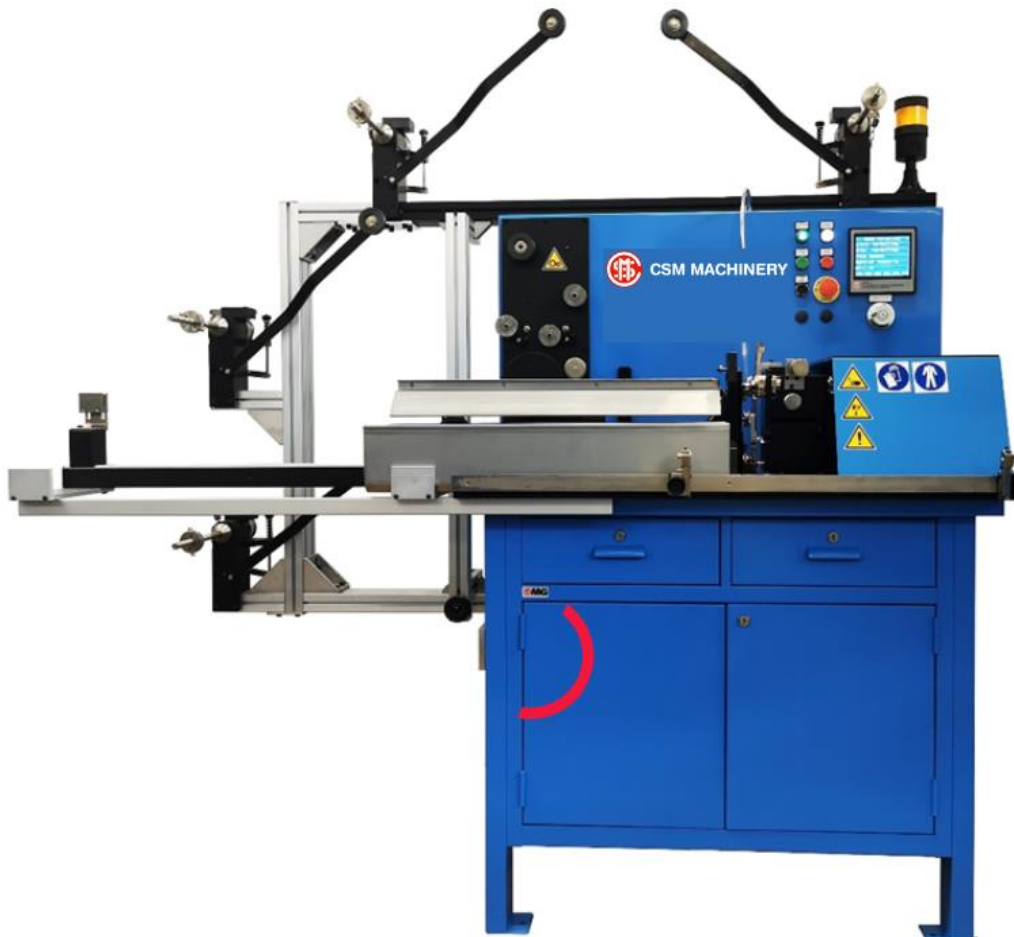
Figure 4 four-wire coiling machine with 4 dynamic brakes
