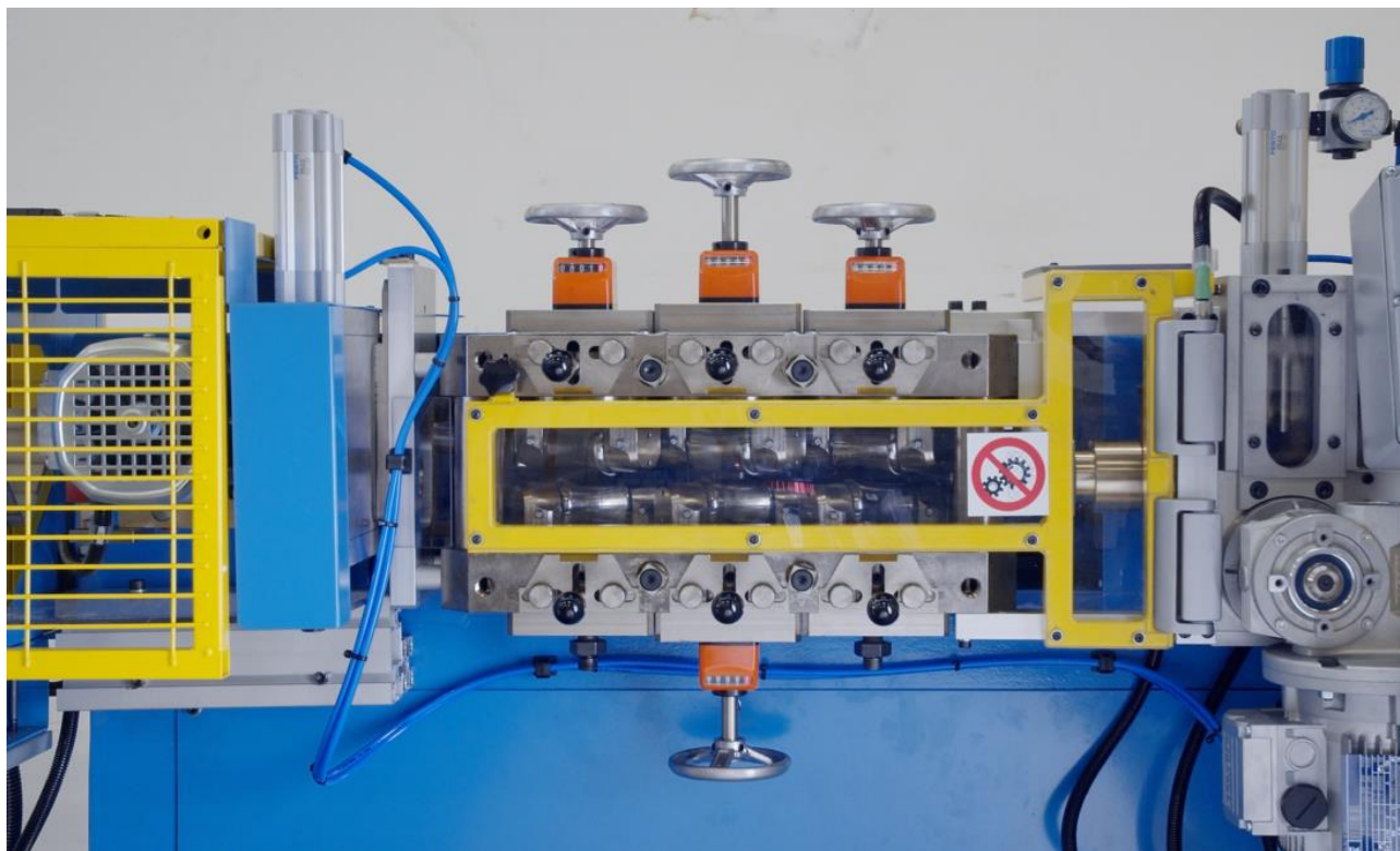
Figure 6 Straightening unit for as welded line
