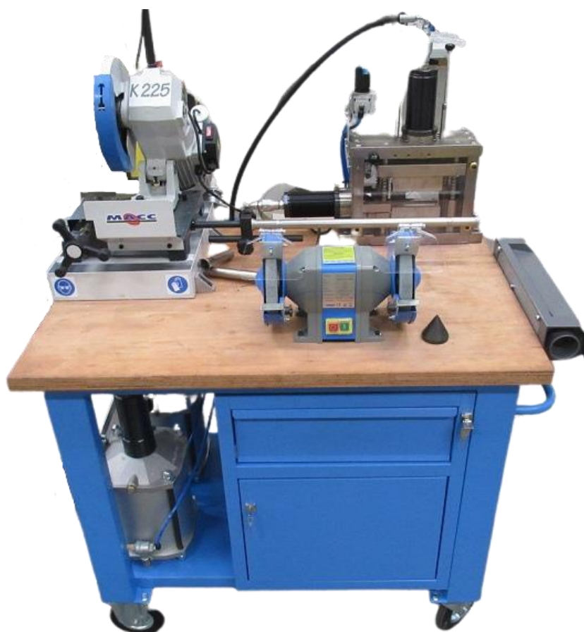
Figure 14 External unit to test the weld quality of stainless-steel tubes
