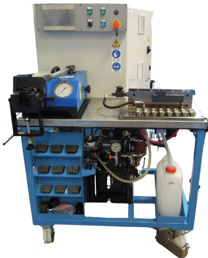
Figure 15 Tube burst testing unit by pressure
