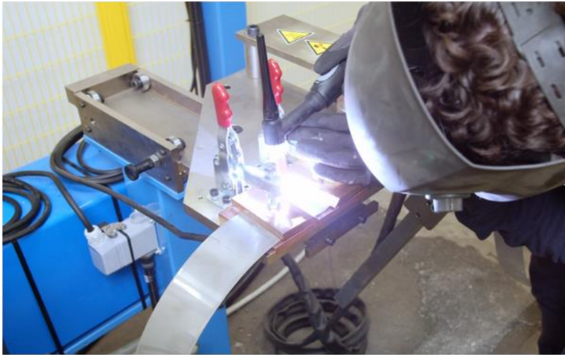
Figure 2 Strip joining bench
