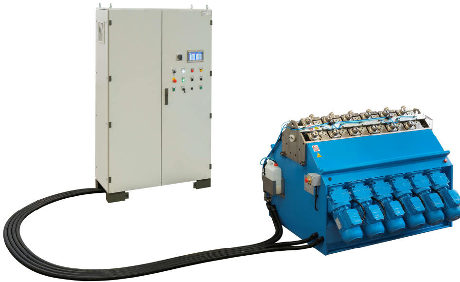
Figure 3: 12-stand roll reducing mill with individual speed control for each pair of rolls and lubricating system
