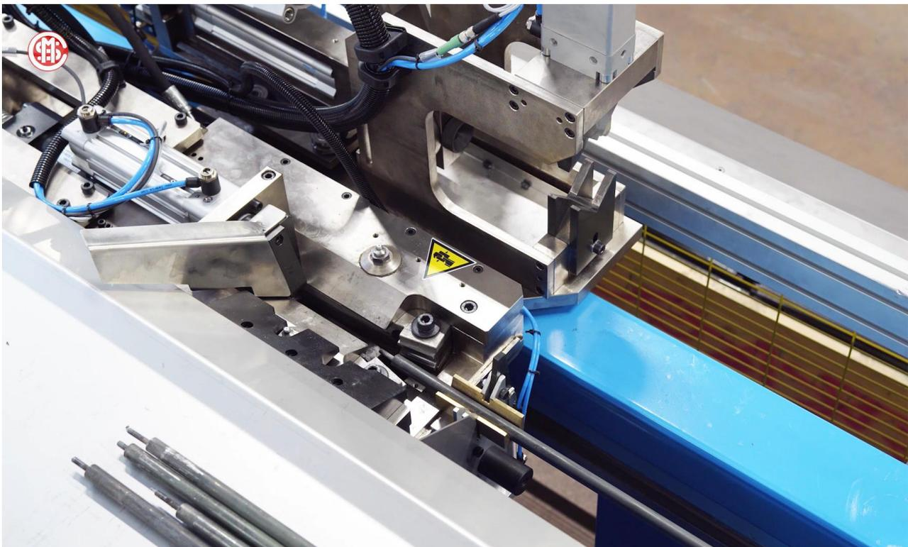
**Figure 1:** Stretching + Cropping of terminal pins to length Mod. 110/95
