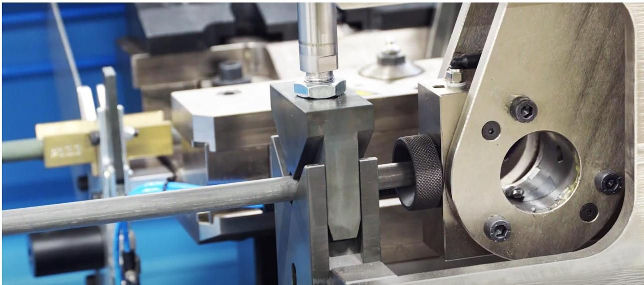
Figure 2: Cropping of terminal pins to length
