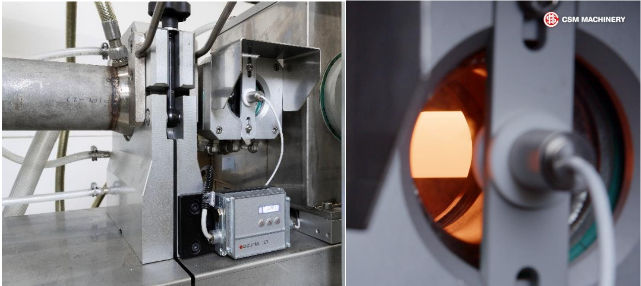
Figure 9 Optical pyrometer to check the tube temperature.
