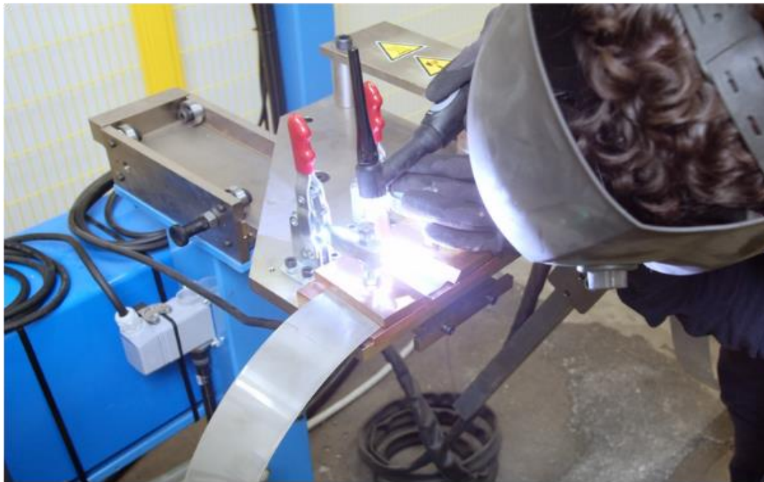
Figure 2 Strip joining bench
