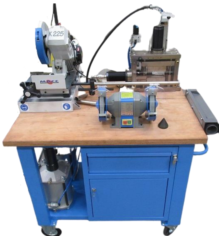
Figure 199 External unit to test the weld quality of stainless-steel tubes
